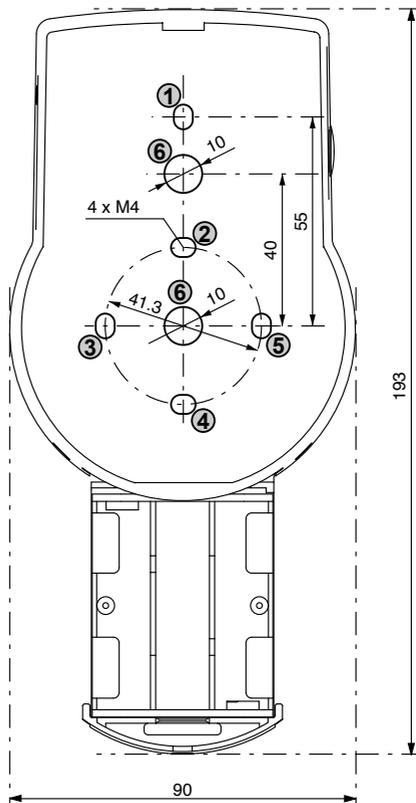
2. Drill the 3 fixation bores  $\text{Ø}3.2 \times 14$  mm and the cable leadthrough bore  $\text{Ø}10$  mm. Remove burrs. Tap M4 threads into the 3 fixation bores.
