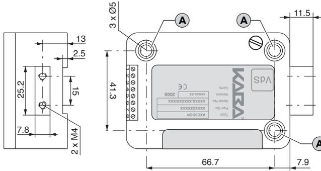
2. Drill the bores  $\varnothing 5\text{mm}$ . Remove the burrs and tap M6 threads into the bores.
