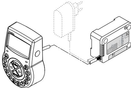
In its standard version the electronic safe lock Axessor USB is battery powered and consist of: the **input unit**, the **lock** and the **connection cable**. The lock includes 2 inputs and 2 outputs (assignment → *External connections at the lock on page 23*). Optionally, an external power supply (6VDC/500mA) can be connected to one of the lock sockets „X1“ or „X2“.
