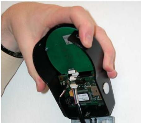
10. Slowly flip down the cover onto the base plate while carefully pulling the connection cable towards the lock chamber; leave some spare loop.
