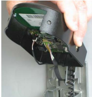
8. Plug the battery cable into the 2 pole connection terminal and the connection cable into the 6 pole connection terminal.
