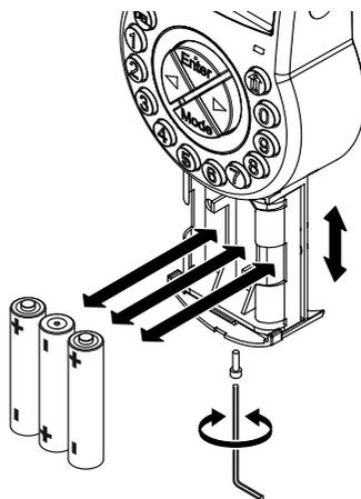
1. Undo the screw of the battery compartment on the bottom side of Input Unit.
